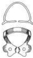
MUH-1680-30 Fig. 00 Narrow jaws for small bicusps. High bow for extra clearance.
