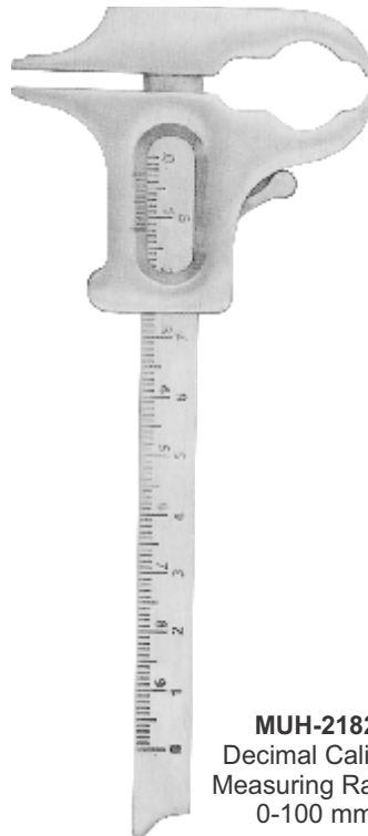
MUH-2182-01 Decimal Caliper Measuring Range 0-100 mm
