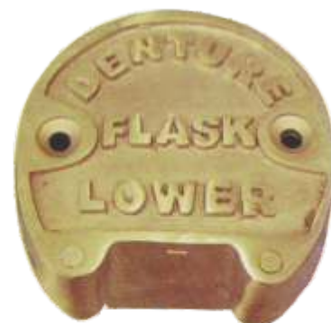
MUH-2240-00 Lower Denture Flask forged Brass Alloy construction. Fitted with Hardened stainless steel Alloy rear Tapered guide pins. Dimension: 4" Long x 3 3/4" wide x 2 1/4" High (10cm x 10cm x 6cm) & weight: 0.920kg
